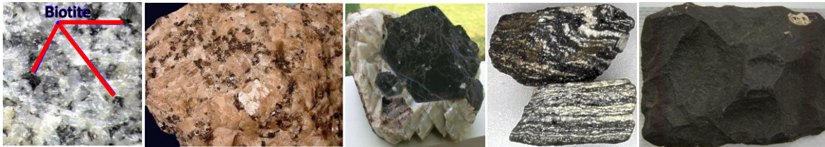
Biotite Mica: in granite Plutonic rocks (3) in pegmatite in gneiss Metamorphic rocks in basalt lava Volcanic rocks
